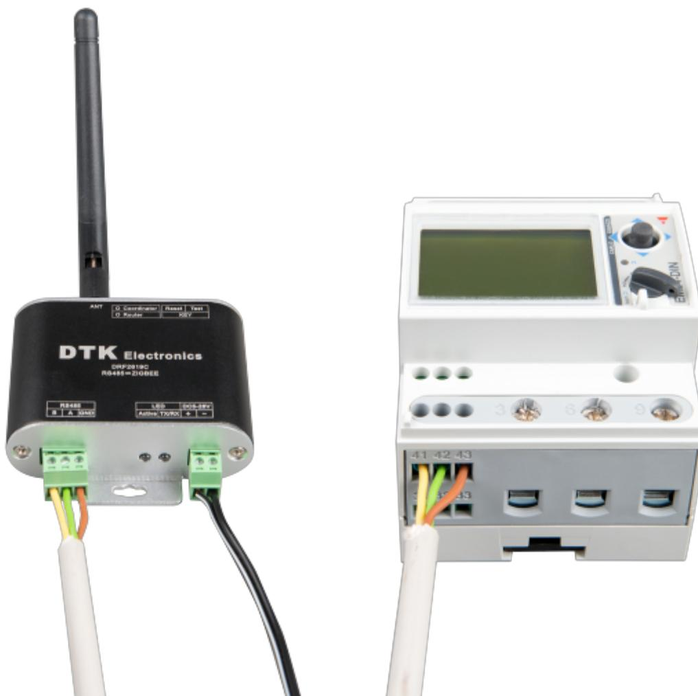
3. Make sure only one Zigbee device is powered up right now: the Zigbee to USB converter connected to the CCGX. Power down all others. *If you don't do this, the Zigbee to RS485 converter may be connected permanently to another Zigbee device.*
